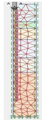
**Figure 7.** Generated mesh in the axisymmetric pile model
