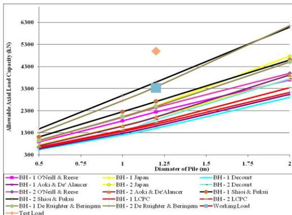
Figure 6. Project 3 – Results by SPT & CPT (D = 32 m).
