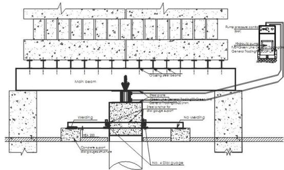
Figure 1. Schematic layout of static axial loading test.
