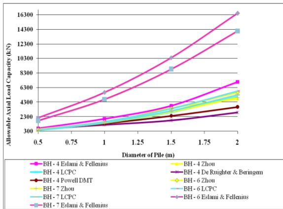
Figure 5. Project 2 – Results by CPTU & DMT (D = 10 m).
