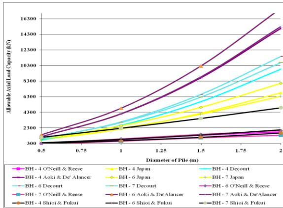
Figure 4. Project 2 – Results by SPT based methods (D = 10 m).
