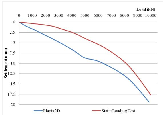
Figure 8. The load – movement curve from PLAXIS 2D from SPT data.
